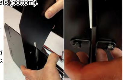
4. Insert 3/4" 10-32 bolt pointing to center then place black lock washer on bolt then hex nut. Fully tighten with 1/8" bit and 3/8" wrench. Check that blade is straight then tighten other 2 bolts.
