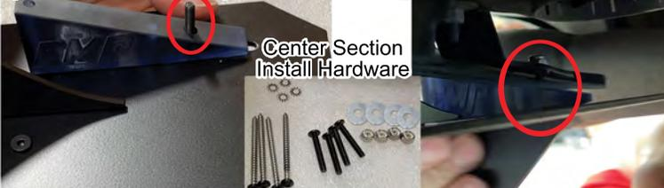
9. You can now adjust the distance of the diffuser center section from the bumper. Hold up so angle spacers will be touching the bumper and ensure tips of the blades aren't touching the bumper. Prop the diffuser in place or have someone hold while the 4 nylock nuts are being fully tightened.
