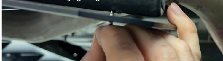
15. Take another shorter install screw and external star washer and install it in the L-bracket hole as shown. Do not fully tighten yet.
