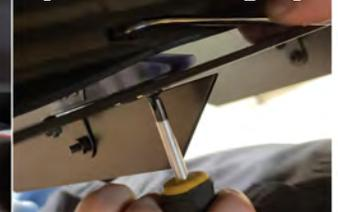
10. Take one of the longer #10 install screws, place an external star lock washer on it, then insert into one of the slots and through a spacer, then screw it into the bumper plastic. Repeat for remaining slots. Do not over tighten these screws! If using a power tool, get screw started then finish tightening by hand.
