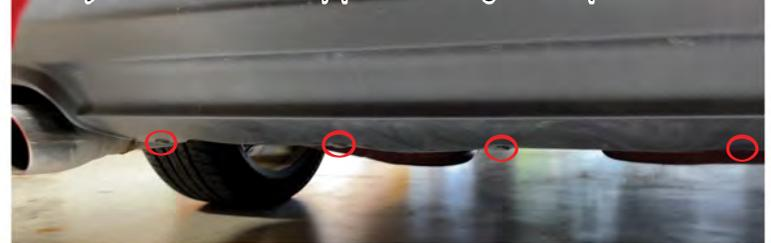
8. Place 1.25" bolt into hole shown on angle spacer from bottom of center section then insert bolt into hole in bumper where plastic rivet was removed. Place a regular washer on bolt then finger tighten nylock nut onto bolt. Repeat for 3 remaining holes.
