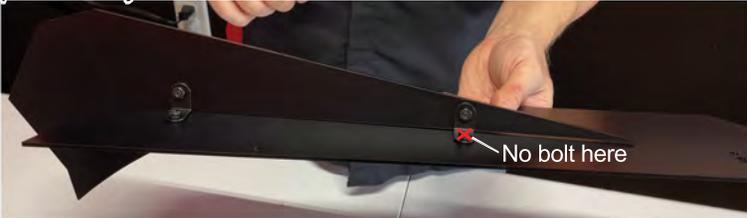
7. INSTALLATION: Remove 4 existing plastic rivets in bottom of rear bumper. They are 2-piece and the bottom piece has to be removed before you can remove the top piece touching the bumper.
