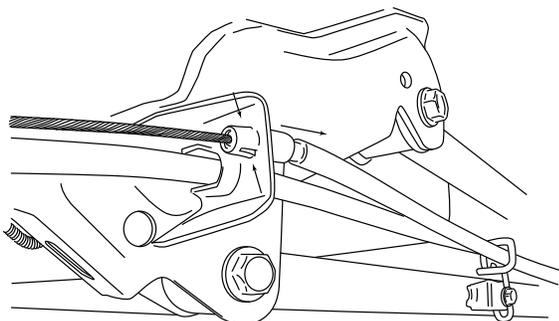
Attach brake cable guide to supplied Brake Cable Bracket (27) and mount bracket with supplied hardware. Reattach brake cable and readjust brake cable adjustment nut to original position.
