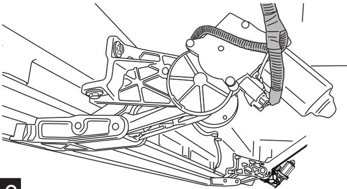
Route wire harness along the upper side of the floor/rocker structure towards to the rear light and rear linkage location. Secure with zip ties (#11). Keep away from exhaust components.
