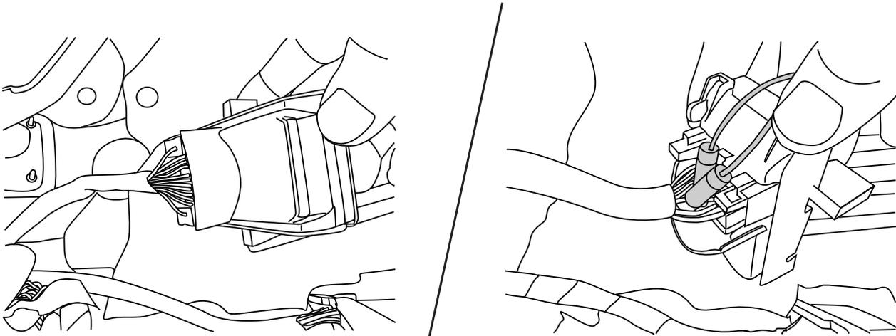
Connect only the purple trigger wire to the OBD II module (#18). Tape off the remaining purple/black stripe wire as it won't be used on this application. Once the trigger wire has been connected to the OBDII module (#18), remove the OBDII port from the vehicle by depressing the two plastic tabs on the sides and push the port back out of the bracket. Now connect the OBDII module to the OBDII port.
