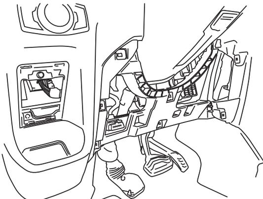
Locate large rubber boot on driver side firewall under the hood. Slice a small opening to run the trigger wire through. Find the trigger wire under the dashboard and strip the wire.
