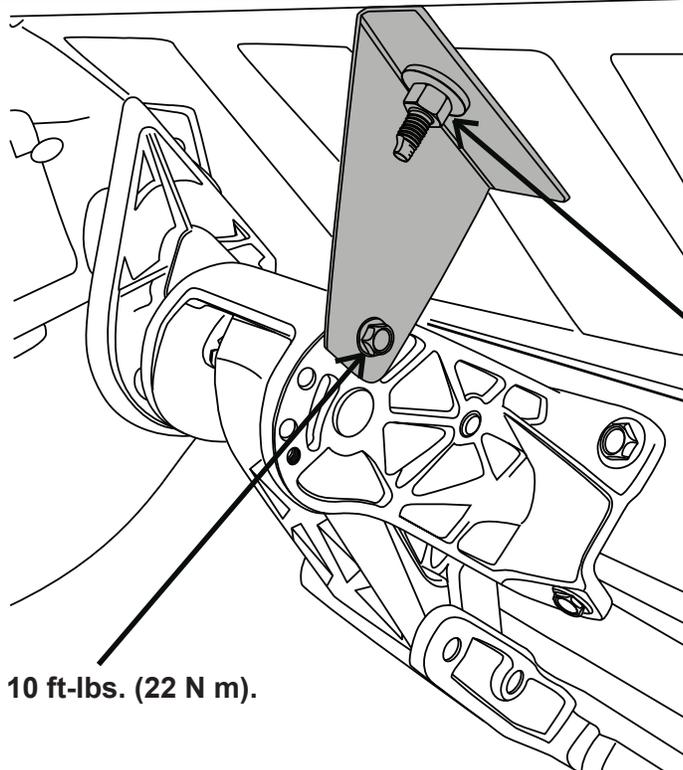
Torque fastener to 10 ft-lbs. (22 N m).
