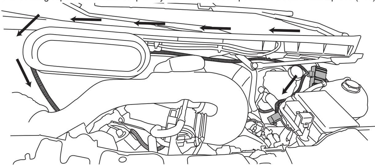
Route wire harness along the upper side of the floor/rocker structure directly towards the front linkage. Secure with zip ties (#11). Keep away from exhaust components.
