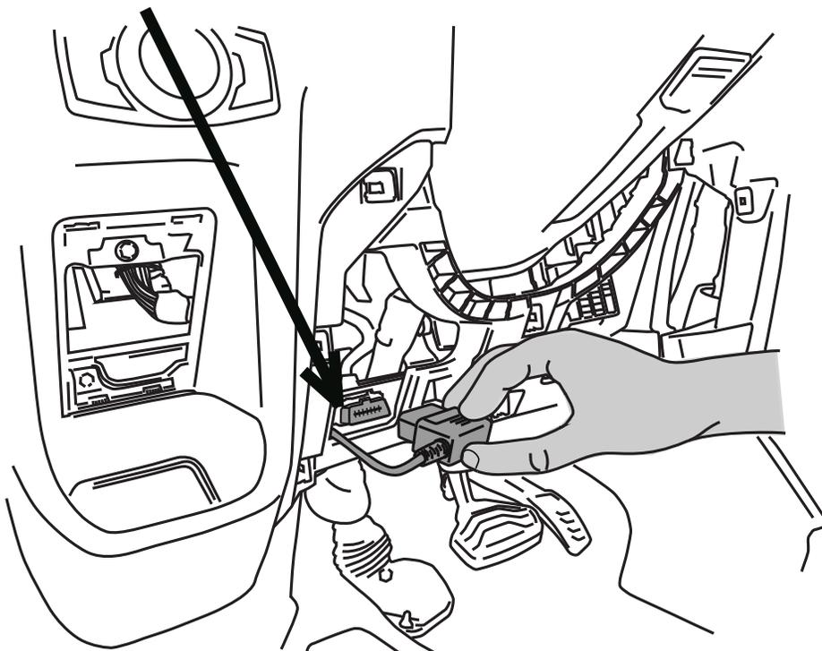
**OBD II install:** Use Supplied Posi-Lock™ (13) connectors to attach the Plug and Play Module to the Harness. Attach matching colors on the harness to the wires on the module. Plug in module to OBD II port on the vehicle. Secure harness with supplied tie wraps. *Note: If the OBD II pass thru harness (76404-01A) was purchased see install sheet supplied in packaging. The pass through harness allows for an open port for other accessories. See below for a brief description.*
