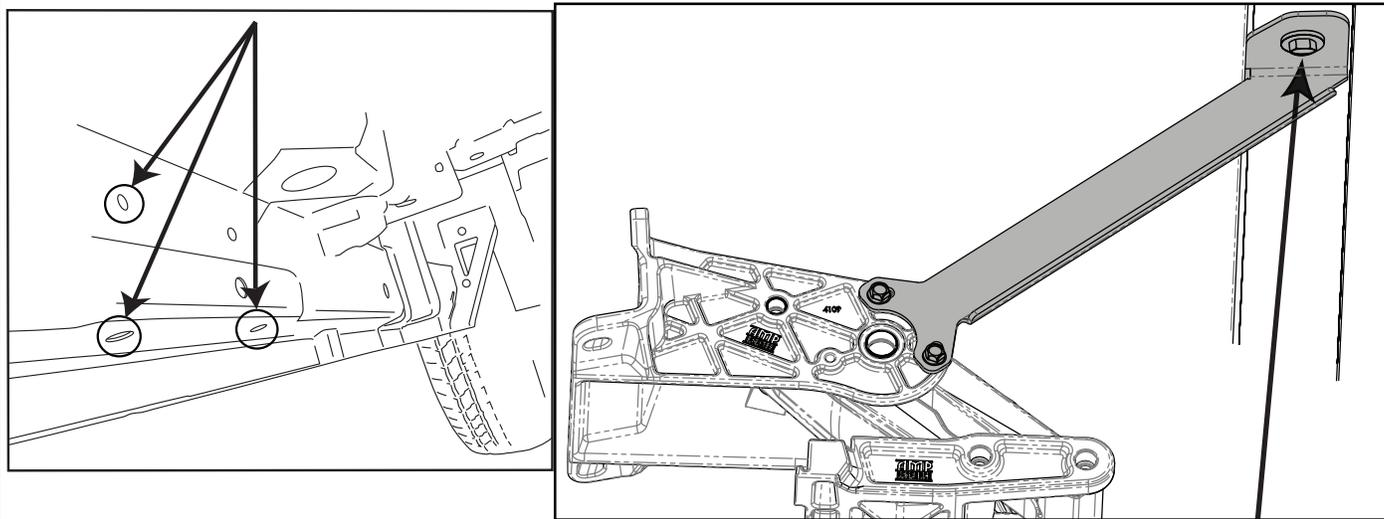
To attach the **Rear Bracket** (#21) to the rear linkage, start by using the Thread Cutting bolt (#23), to cut threads in the blank insert in the frame rail. Use a 9/16" socket and ratchet, go slow and stay straight. Then install the bracket on the non-motor side of linkage loosely with two bolts(#22), install the upper Bolt (#23) and Washer (#24), loosely and tighten the bottom two bolts fully. Now, tighten the top.
