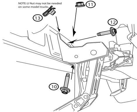
Slide mounting T-nut into position, aligning the end of the board with the rear edge of the back door. Mount board and tighten fasteners to 10 ft-lbs. Insure linkages are squared to body prior to torquing fasteners.
