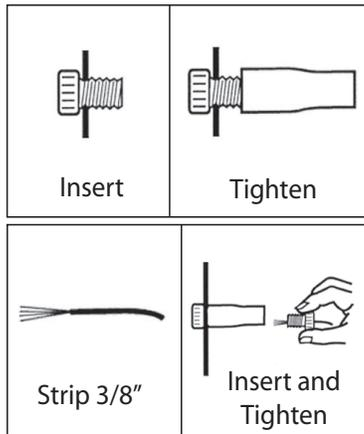
Using supplied Posi-Tap connector connect trigger wire on harness (Driver Side: Grey/Black Stripe & Passenger Side: Tan/White Stripe) to Solid dark grey wire on door switch plug. Passenger side shares the same color wire. **Note: Wire is located in the upper outer pin of plug. (Left on Driver, Right on Passenger Side)**
