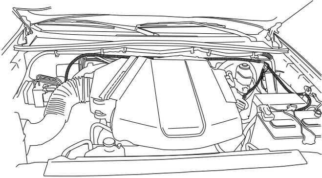
**12** Note: Run loom with Green/Yellow and Pink/Black Trigger wires down drivers side of vehicle.
