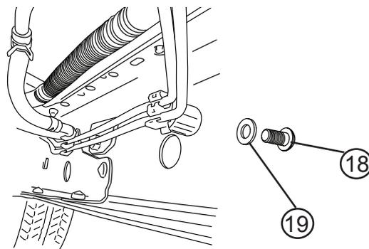
Replace all brake line fasteners.
