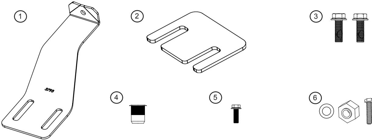
For Dually applications install provided brackets and spacer between linkage assembly and lateral bracket. Use supplied M10x40 bolts. **Do not tighten bolts yet. Continue with installation provided with p/n 75406-01A.**
