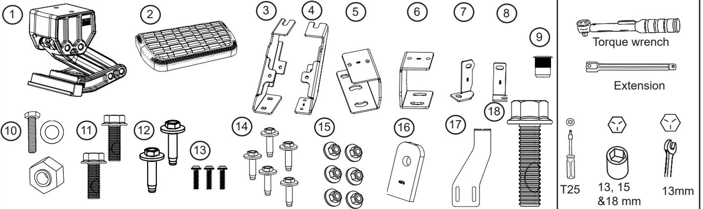
Components must be configured for Passenger or Drivers-Side as shown.
