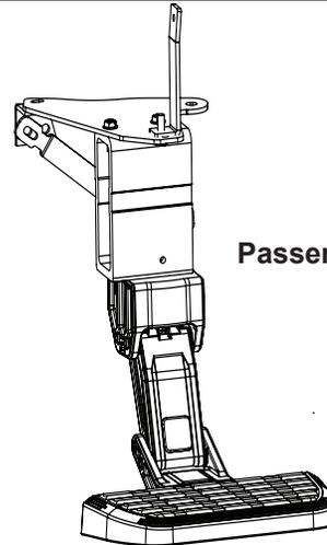
Using a 12mm socket or wrench loosen both brake cable brackets. **Note: Passenger side only has one bracket to remove.**
