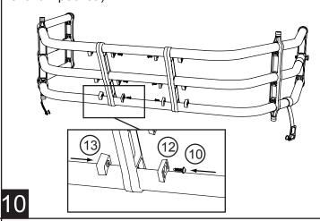
Adjust bumper uprights so that the bumper rests on a flat surface on the tailgate.
