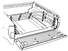
When MOTOXTENDER is out on the tailgate be sure to fasten strap latches properly.
