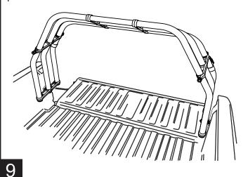
Secure the center uprights with double wedges and PT screws. (The thru-hole wedge is placed in the shallow pocket.)
