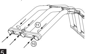
Install strap latch retainers and end caps.
