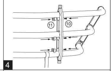
With the assembled arranged as shown (tube ends should extend through the pivot upright approx. 3/8"), secure pivot upright with large wedges and PT screws. Torque to 20 in-lbs.
