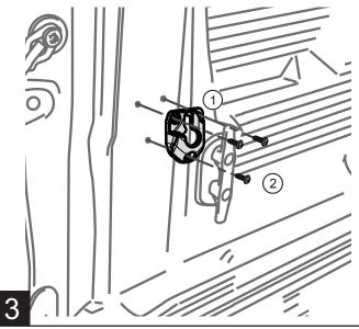
Fasten mounting brackets using the Phillips head screws and torque to 30 in. lbs. If equipped with bedliner, install mounting brackets over bedliner.
