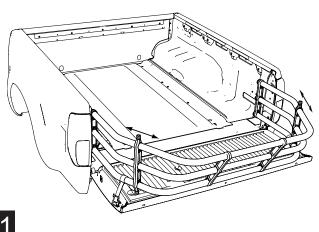
Rotate MOTOXTENDER into the bed to check that the bumper position is on a flat surface. Torque PT screws to 20 in. lbs. Close tailgate and check for clearance.
