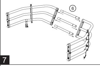
Connect the two halves. Make sure there is a minimun of 3" of overlap with the bent tubes on each half.
