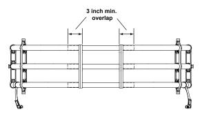
\*For truckbeds narrower than 54" (between D-pillars) cut 2" off of each end of straight tubes.
