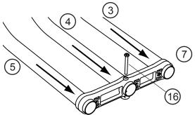
Insert Phillips screw through pivot upright and predrilled center tube. Torque screw to 18 in. lbs.
