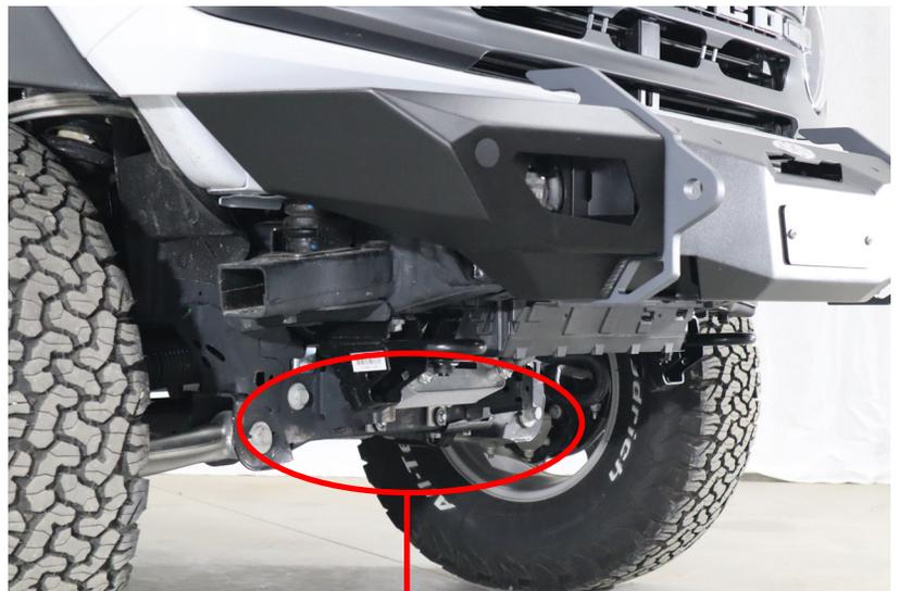
You will need the two black bolts that were used to hold your stock front air dam or skid plate located here.
