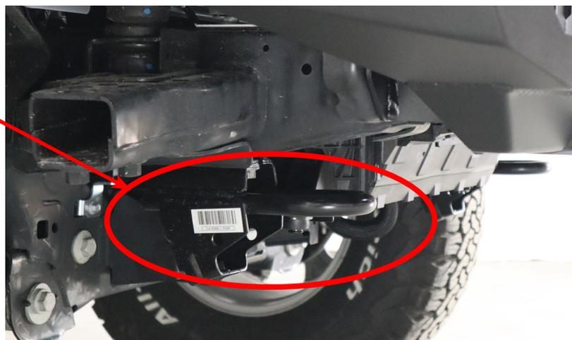
Only remove one bracket at a time so the Intercooler does not drop.
