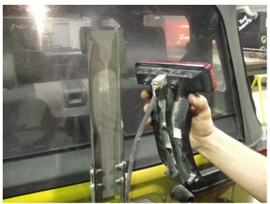
3. Plug the factory light back into the harness plug.
