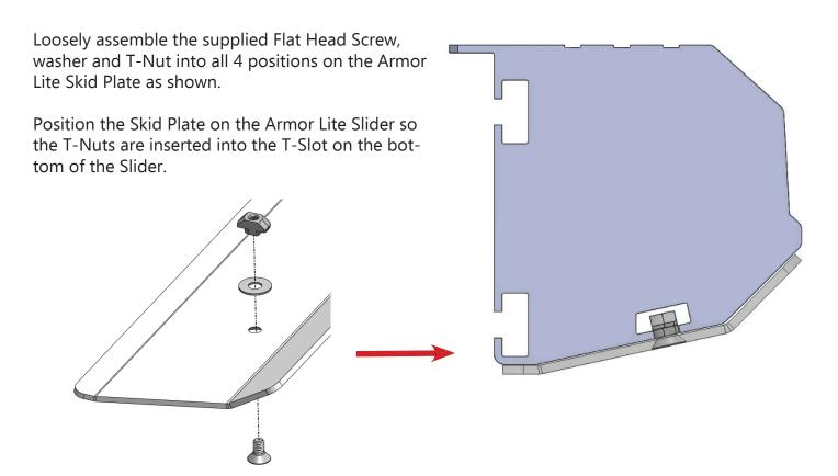
Using a Allen wrench, turn each Flat Head Screw 90° clockwise so that the shoulder on the T-Nut catches on the T-Slot as shown below.
