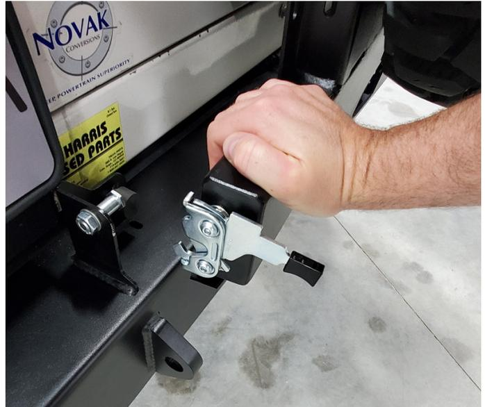
With the swing arm closed, unthread the small rubber bumper until it touches the arm, then add another 1/2 to 1 full turn. This bumper should limit the Swing Arm movement and keep the Latch from rattling against the Striker Bolt.
