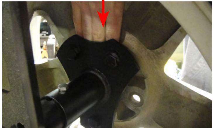
Your tire should squeeze against the back plane of the tire carrier at the top and the bottom.
