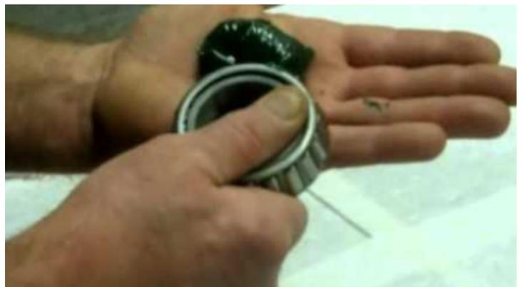
Next place the tire carrier Swing Arm upside down as shown in the image below. Insert the greased bottom bearing LM29749 into the housing with the tapered side facing into the housing.
