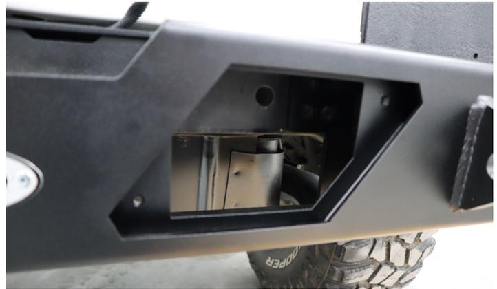
Install the 7/16" Hex Bolts, Washers and Frame Backing Plate as shown into the holes that you drilled into the rear Cross Member. With the gas tank skid plate lowered as shown, you will be able to insert the Frame Backing Plate behind the Cross Member. You can access bolt holes thru the light bezel opening in your bumper.
