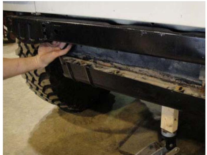
Install the Bottom Bracket as shown using 7/16" Hex Bolt and washers into the bumper, and the supplied metric M12 Hex bolt and washer into the frame.
