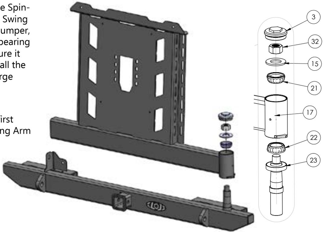
It is a good idea to add a little blue loctite to the Nut to prevent loosening. Slowly tighten the nut using a 1-1/2" Socket. Check the swing arm movement every 1/8th turn. The Swing Arm movement should not be restricted and should move freely. Overtightening could damage the bearings.
