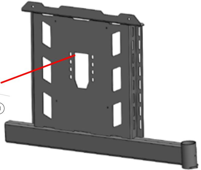
With the tire mounted, there could be a small gap between the back of the wheel and the Tire Mount Plate approximately 1/4"-1/2". This is ok because the tire is pressed against the Tire Carrier Back Plate. The tire should be tight against the back plate and not able to wiggle side to side or up and down. This keeps the tire from shaking on the tire carrier.
