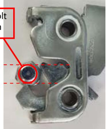
Next position the latch on the X-Axis using the Latch Spacer and/or the 1/4" washers to position the head of the Striker Bolt as close to the BLUE highlighted face without rubbing.
