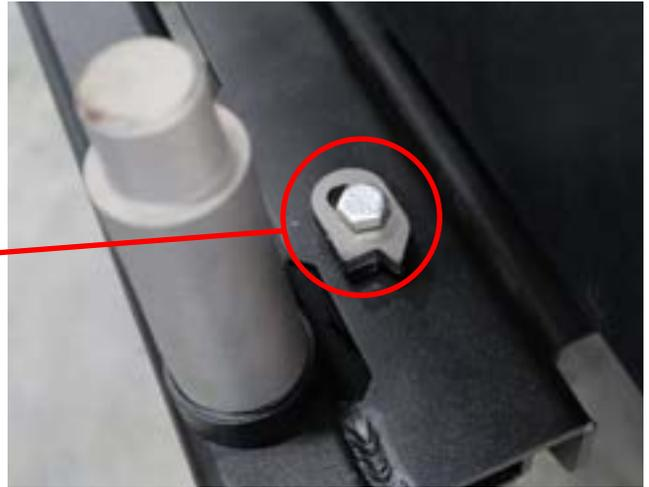
\*\*\*The Swing Stop is designed to allow the swing arm to rest in the open position when the Jeep is out of level. It is also a safety feature that will help stop the tire carrier Swing Arm from swinging around and damaging your Jeep. Repeatedly allowing the Swing Arm to swing around uncontrolled could damage the swing stop. Always open the Swing Arm and allow it to gently rest against the Swing Stop.\*\*\*
