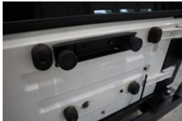
Install the Bumper Door Bracket so the two large bumpers line up with the ribs on the back of the tire carrier Swing Arm. Adjust the Bumper Door Bracket as needed and tighten securely.
