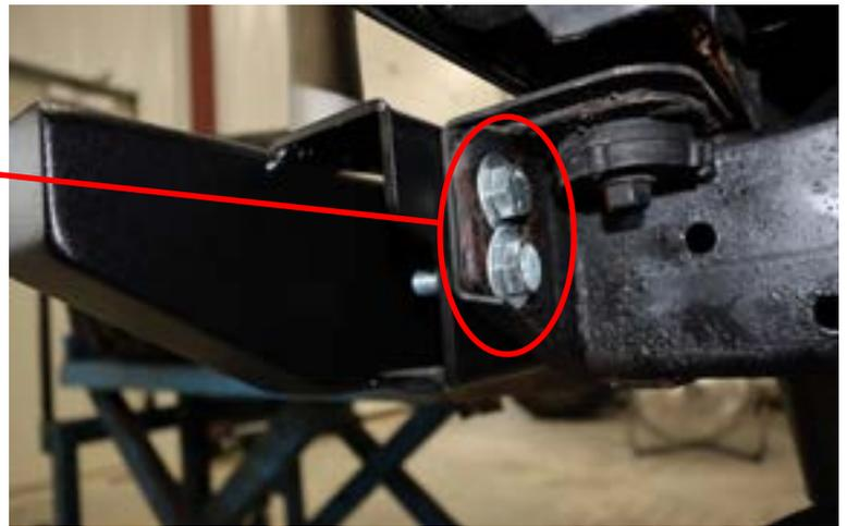
Install the 7/16" Hex Bolts, Washers and Frame Backing Plate as shown into the holes that you drilled into the rear Cross Member. With the gas tank skid plate lowered as shown, you will be able to insert the Frame Backing Plate behind the Cross Member. Leave these bolts loose while you finish the bumper installation.
