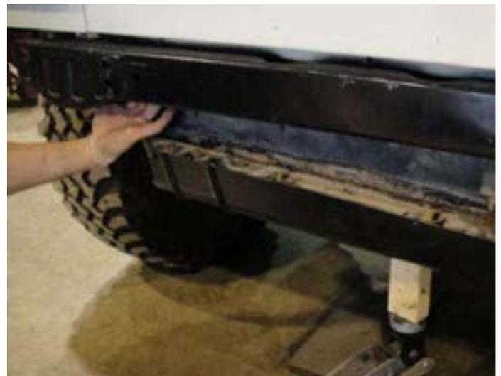
Install the Bottom Bracket as shown using 3/8" Hex Bolt and washers into the bumper, and the supplied metric M12 Hex bolt into the frame.
