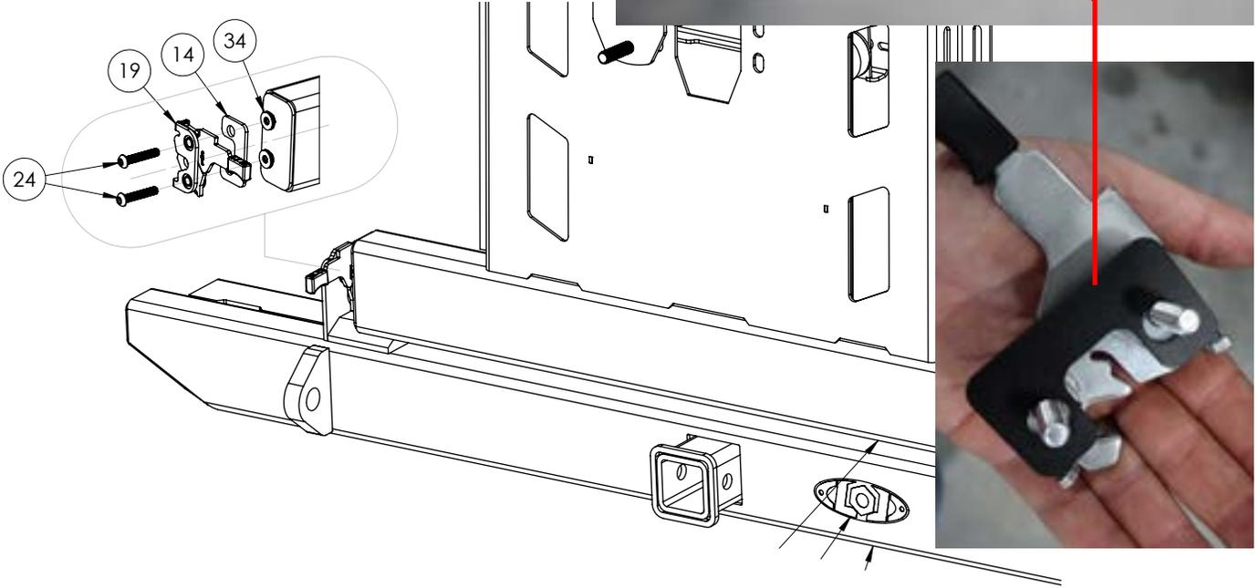
Next install the Striker Bolt with Yellow Zinc plated Washers and Metric M10 Nut. Just snug these up for now until all adjustments are made. Also install the small rubber bumper as shown.
