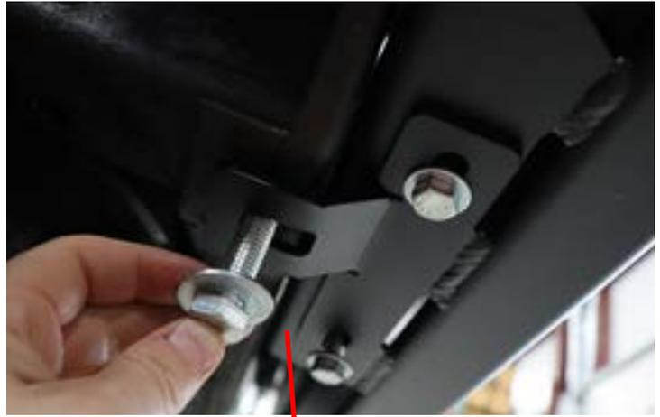
Once all the bolts are installed, make sure the bumper is centered on the Jeep and level side to side. Tighten all the mounting bolts securely. Once the bumper is secure reinstall the gas tank skid plate.
