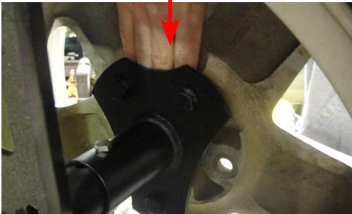
Your tire should squeeze against the back plate of the tire carrier at the top and the bottom.
