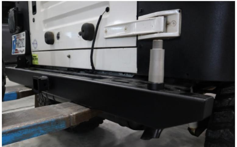
Install the 7/16" Hex Bolts, Nuts and Washers into the two outside mounting holes first. Leave these slightly loose while you finish the bumper installation
