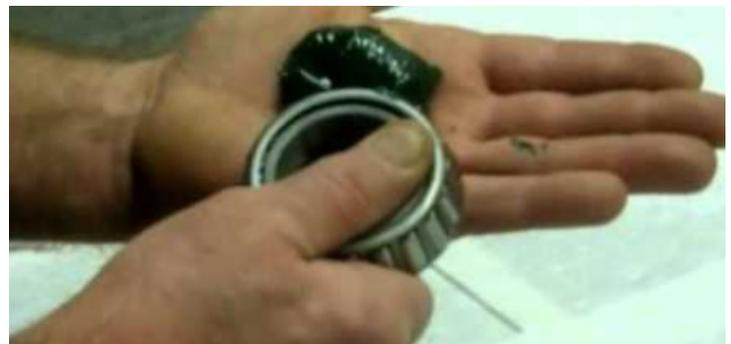
Next place the tire carrier Swing Arm upside down as shown in the image below. Insert the greased bottom bearing LM29749 into the housing with the tapered side facing into the housing.
