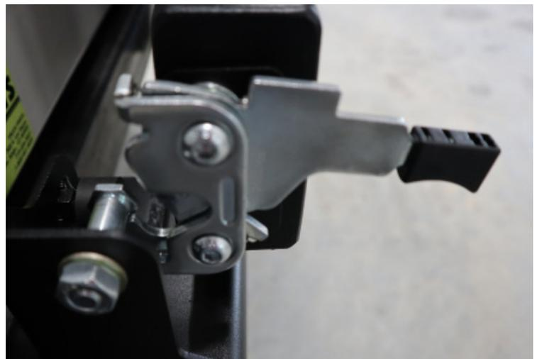
Always close the tire carrier Swing Arm by pushing on the arm near the Latch or the bottom of the tire. This helps to insure the Latch catches the Striker Bolt securely.
