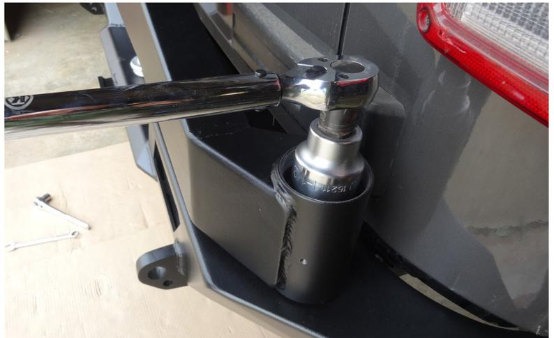
Install the tire carrier Swing Stop. Be sure to adjust it to allow the Swing Arm to open completely and allow full use of your tailgate and tighten securely. If you have accessories mounted on your tire carrier, you can adjust this slightly to help avoid the accessories hitting the Jeep when you open the Swing Arm.
