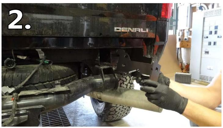
SLIDE THE FRAME MOUNTS INTO THE FRAME RAILS. ORIENT THE MOUNT AS SHOWN IN THE PICTURE ABOVE.
