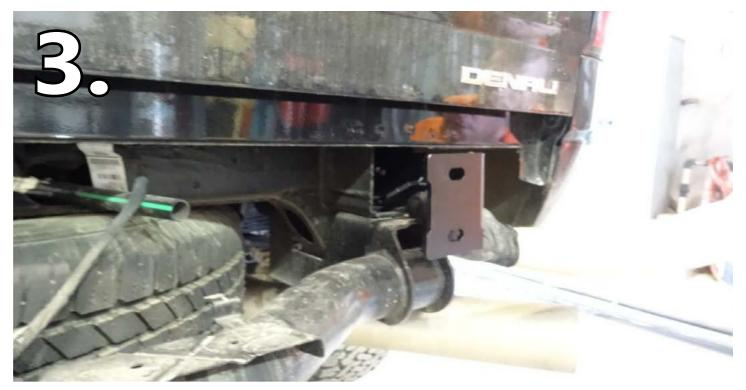
THE NEW FRAME MOUNTS WILL BE BOLTED ON THE INSIDE OF THE FRAME RAILS BUT TOWARDS THE OUTSIDE OF EACH RAIL. THE MOUNTS WILL HAVE THE BENT PARTS FACING TOWARDS THE MIDDLE OF THE TRUCK.
