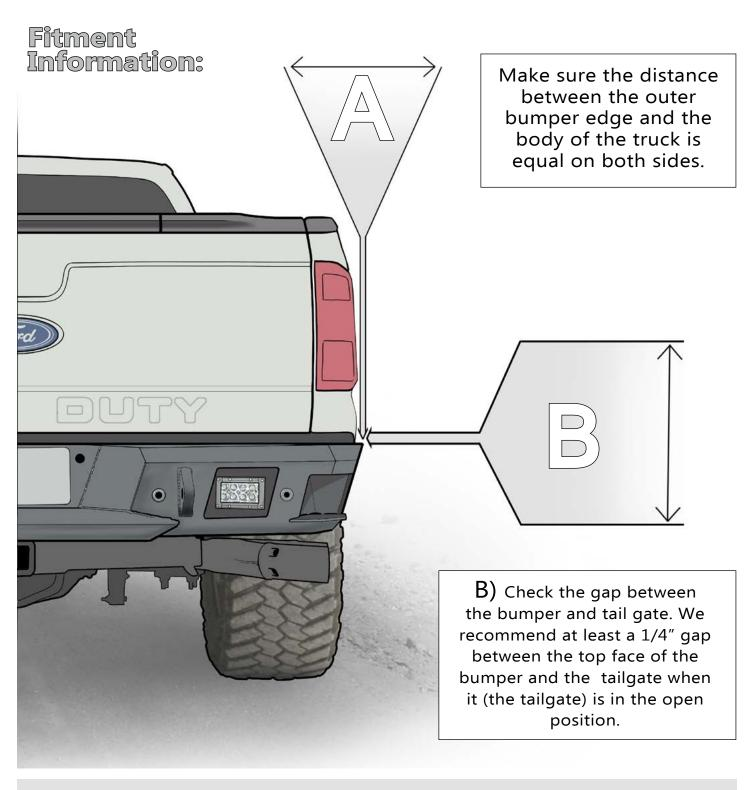
Align bumper in the horizontal and vertical directions, making sure that it is level.
