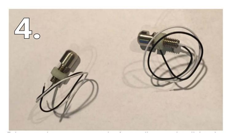
The lod bumper does not support the factory license plate lights. We offer replacement bolt lights.
