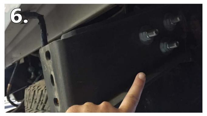
Install the replacement rear mounting brackets on the driver and passenger sides of the frame. use the three 1/2" bolts and nuts provided as shown.
