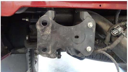
2) Also remove these brackets from the rear of the frame. Keep the four small bolts from these mounts because you will need them to re-mount the new bumper.
