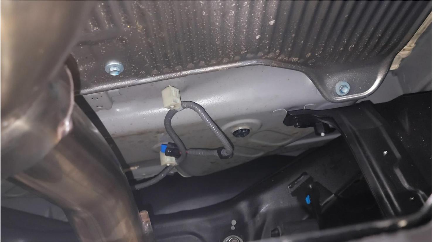
**Step #4** – Secure the electronic valve connector in a safe spot away from any moving components.
