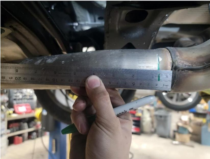
**Step #2:** Use a Sawzall to cut the factory exhaust.
