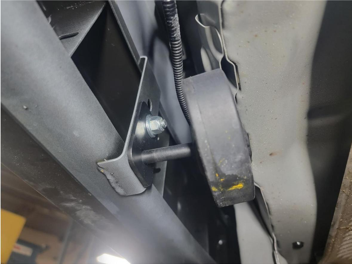
**Step #3** – Slide the exhaust hanger located over the tips into the newly installed rubber isolator. (Circled in green below)
