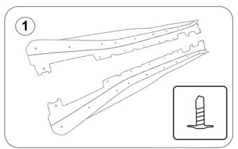
1.- Parts received in this package:1x ZL1 Side Skirt set36x self tapping screws
