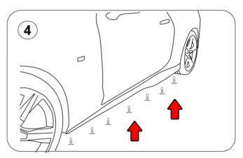
4.- Finish the installation by mounting the desired number of self tapping screws to the sideskirt.
