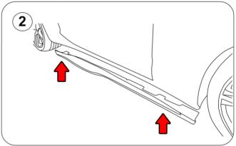
2.- Mount the sideskirt into it's respective place. Use any tools necessary to hold it in place.
