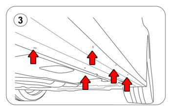
3.- According to the predrilled holes, drill the necessary holes wanted for the installation. if you don't drill the 18 holes, you can use double sided tape to improve the support toughness.
