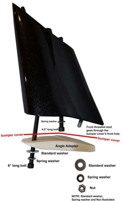
NOTE: Standard washer, Spring washer and Nut illustrated above secures the threaded stud from underneath the adapter.
