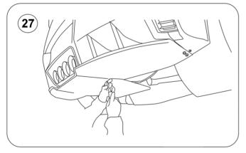
27.- Screw the 7 allen bolts that correspond to their respective pre-drilled holes, making sure to also tighten the bolts for the T-mounts.
