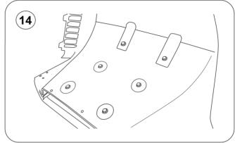
14.- Secure the plates against the diffuser using the set of hex bolts and washers provided.
