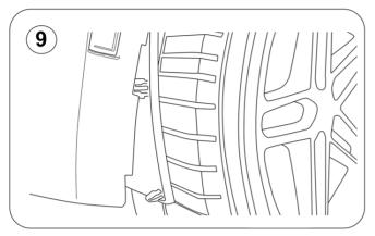
9- Pop out the tabs on the splash guards behind the rear tires. Afterwards remove the torx screws beneath the splashguard.
