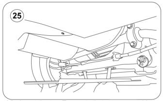
25.- Insert the two T mounts that were assembled on **step 18**.
