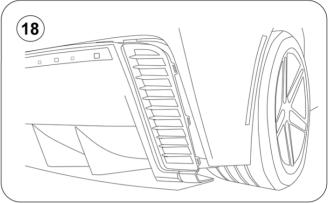
18.- Re-attach the vent tabs on to the diffuser.
