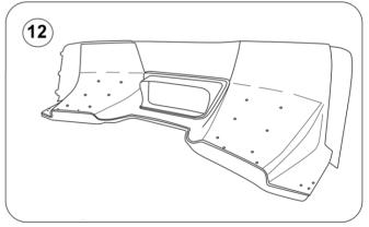
12.- Drill the 12 holes on the diffuser that correspond to the undertray's pre-drilled holes.
