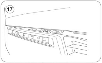
17.- Re-attach the tabs making sure they snap in with the bumper fascia.
