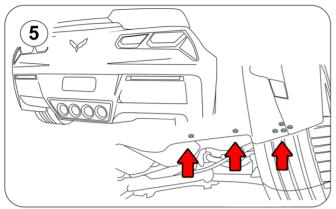
5.- Locate all the screws at the bottom. **NOTE**.- OEM hardware will be re-used to reinstall the diffuser later on.
