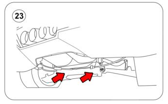
23.- Locate the "Rear Crossmember subframe", the T shape mounts are going to be mounted on the holes that are present in this subframe.
