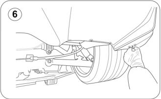
6.- Use any tools at your dispossal to safely remove the screws. A size 7 socket is recommended for removal
