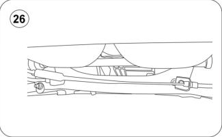
26.- When the T shape mounts are inserted all the way through, rotate them 90 degrees so the extensions on the T mounts rests directly on top of the subframe's top outer surface.
