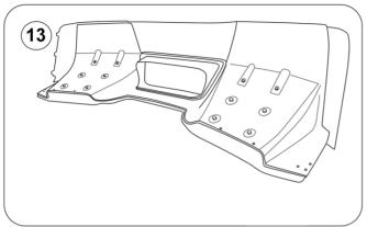
13.- Place the reinforcement plates behind the diffuser, matching up the plate's pre-drilled holes with the holes previously drilled on the diffuser.
