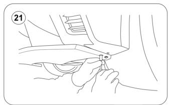
21.- Screw back the OEM bolts previously removed making sure that the undertray's pre-drilled holes match up with the vehicle's factory mounting points.
