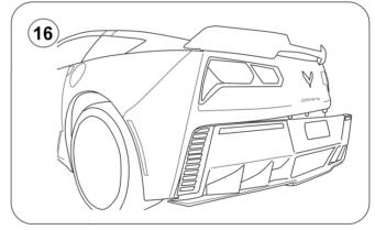
16.- Snap the diffuser back in place, making sure that all the diffuser's upper tabs line up propertly with the rear bumper fascia's slots.
