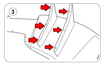
3.- Add marking material on the predrilled holes.
