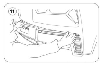
11.- Remove the diffuser starting from one side to another by gently pulling the tabs located above of the diffuser.
