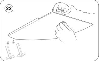
22.- Place the T shaped mounts behind the pre-drilled holes of the undertray's attachment, use a flat allen screw to secure the mount. Note.- Do not fully tighten the bolt until the mount is fully assembled with the vehicle.
