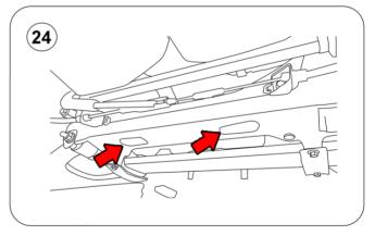
24.- Locate the two holes that are going to act as a mounting support.
