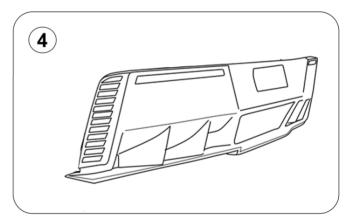
4.- With the diffuser mounted on the car, place the undertray to mark mounting points to be drilled on the diffuser.
