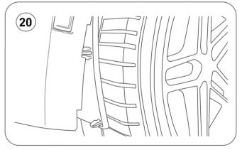
20.- Re-attach torx screws and splash guards.
