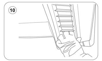
10.- Use both hands to gently remove the vent by pushing it from the inside aperture where the splash guard was located.
