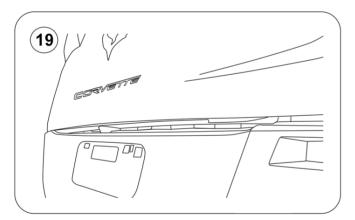
19.- Make sure to screw the bolts previously removed after snapping in the diffuser.
