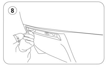
8.- Remove the bolts that are located behind the reflector as well as the bolts located inside the exhaust area and behind the license plate.
