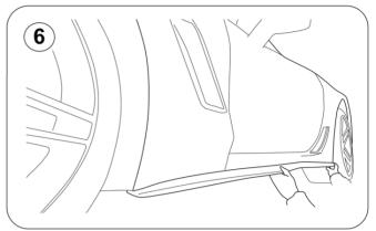
6.- Bolt the side skirt, using the factory bolts previously removed.
