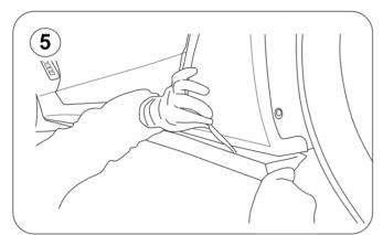
5.- If double sided tape is being used as an additional gripping method. Make sure to stick the side skirt on to the rocker panel before fully tightening the bolts at the bottom.
