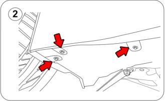
2.- Remove the 3 size 7 bolts located underneath the front fender.
