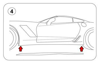
4.- Place the side skirt, matching up the side skirt's pre-drilled holes with the vehicle's factory mounting points.
