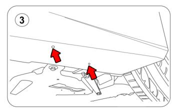
3.- Remove the 2 bolts located at the rear of the rocker panel.
