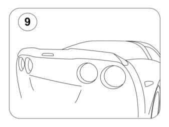
9.- Once the Rear Spoiler is properly attached to the vehicle. Reinstall the brake lights re-using the OEM hardware.
