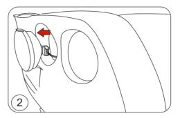
2.- Remove the four brake lights from the car.
