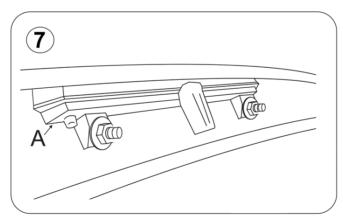
7.- Secure the brake lights with a nut and washer.
