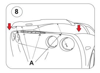
8.- You will need to drill a hole on each side of the bumper (Section A) to match the pre-drilled holes on the Rear Spoiler outboard. Test fitment/placement is recommended before drilling, using a piece of chalk or crayon inside the spoiler pre-drilled holes can help mark the correct drilling spots on the bumper during the test placement.
