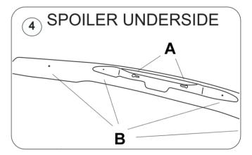
7.- Locate the 4 predrilled holes (B) underneath the spoiler, also locate the two holes (A) that will secure the nuts that are used to mount the brake light.
