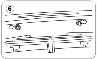
6.- Carefully mount the brake lights into the spoiler making sure you allign the screws into the brake light mounting points.
