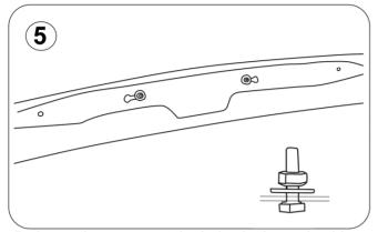
5.- Insert the screws at the holes in the underside of the splitter with the head of the screw facing inside, secure the screw with a nut and washer.
