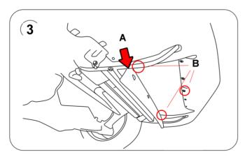
3.- Locate the middle air dam and remove it from the car by unscrewing the two bolts located at each side of the air dam (A), this part is removed to facilitate the removal of the two screws that are located in front of the air dam screws.
