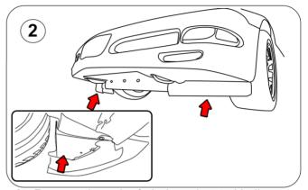
2.- Remove the pair of air dams located bellow at the front bumper fascia, Then remove the Plastic liners behind the pair of air dams.
