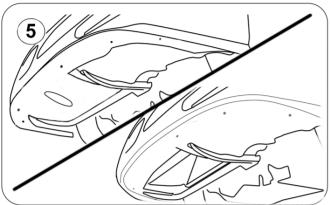
5.- Using the Splitter's pre-drilled holes as guidelines, mark the front bumper fascia with any marking material. (double-sided tape can be used to temporary mount the splitter to the front bumper fascia)
