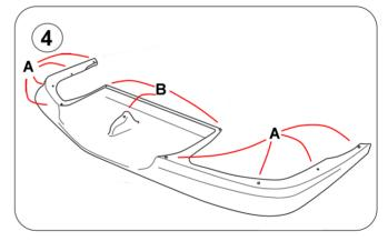
4.- Locate the 8 pre-drilled holes that are situated on the splitter's inner flange (A) these holes will serve as a template to mark the drilling points on the front bumper fascia later on.
