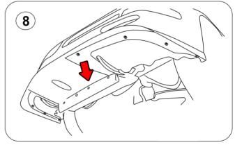
8- Finish the installation by mounting the previously removed middle and side air dams.
