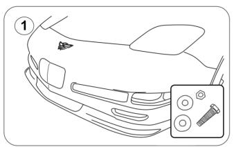
1.- Parts received in this package:1x ZR1 Style Vented Front Splitter for C58x Hex bolts8x 1/4" x 20 nuts16x Washers
