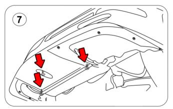
7.- Place the 3 OEM screws that are located on the center and the rear of the splitter's under tray
