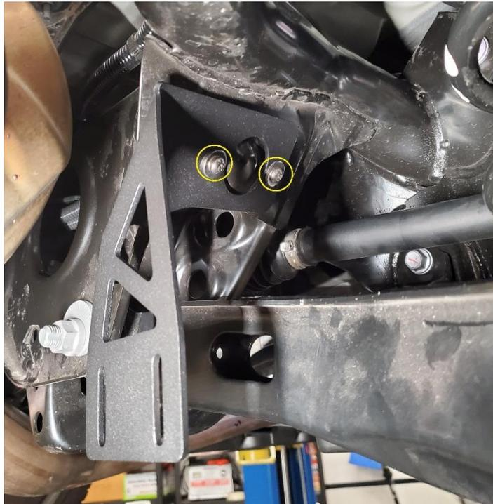
**2.5.** Locate, and remove the clips for the C-shaped bracket installation. The passenger side is shown below. The driver side is a mirror.
