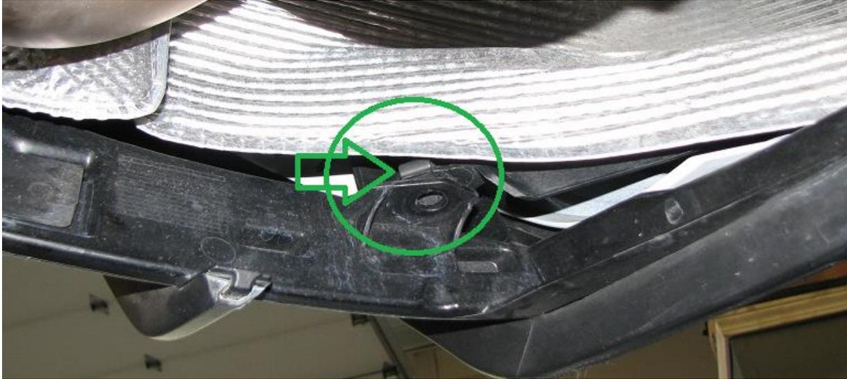
**2.11.** Finally, remove the T30 bolt circled in orange in step 2.4 and the below image.
