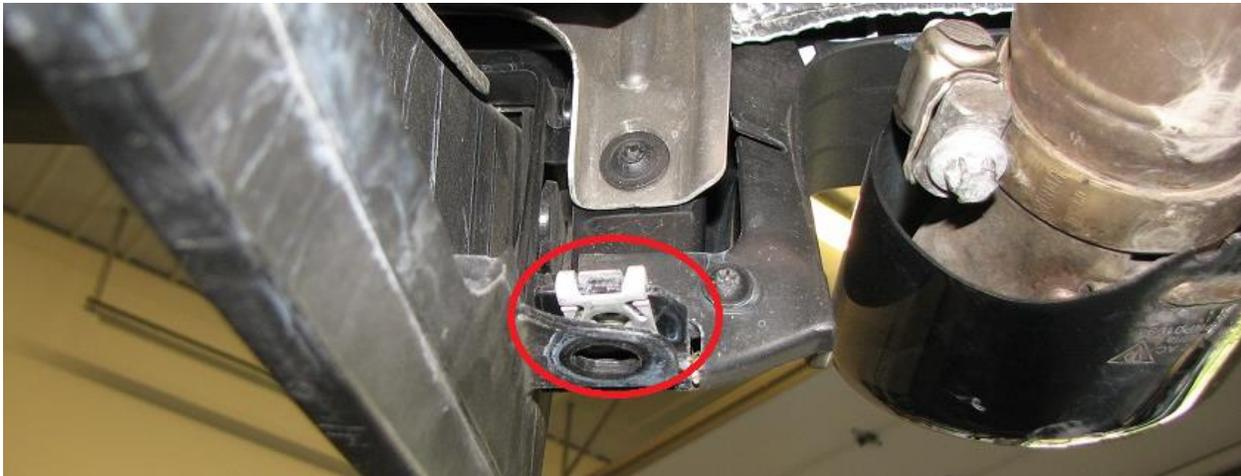
**2.8.** Remove the T25 bolt shown below, circled in blue in both step 2.4 and below.
