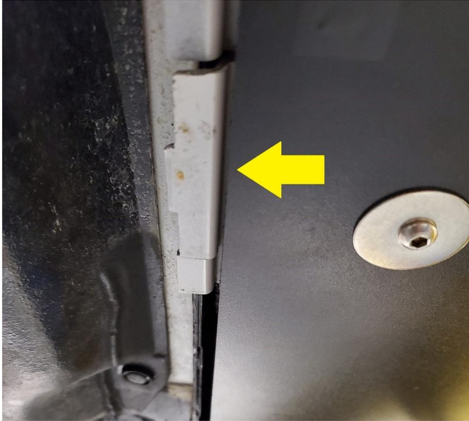
2.5. Holding the side splitter still, mark each slot.
