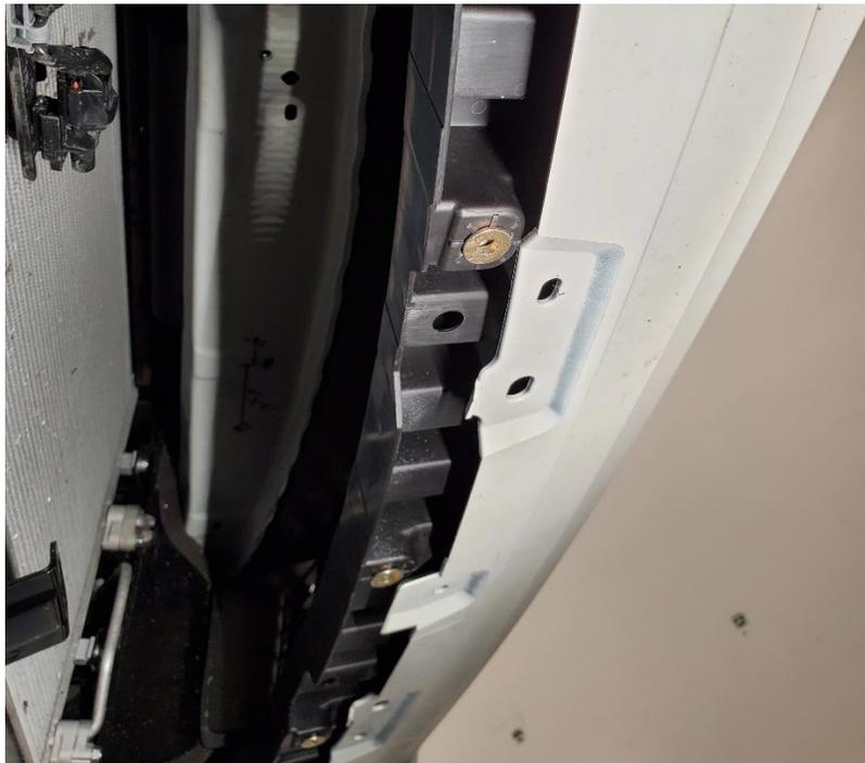
**2.14.** To install the splitter rods we will need to measure the point to drill for rivet nut installation. Looking upward at the crash bar, locate the two slotted holes.
