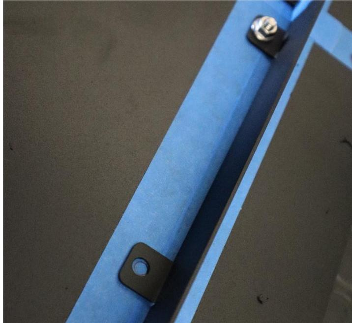
**3.9.** Drill the bolt holes with a 1/4" drill bit.
