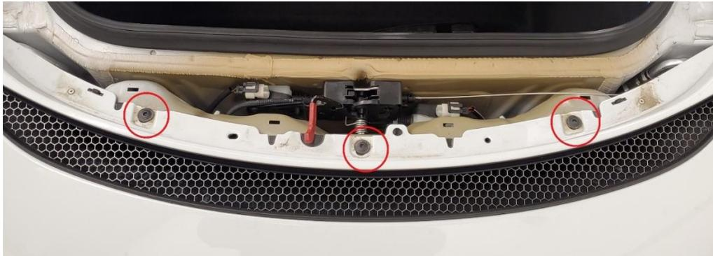
**2.10.** Using a small hook completely pull out the bumper release tabs on the inside of the headlight housing.
