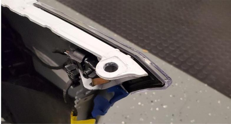
2.6.1. Disconnect the electrical connector on both sides, and the headlight washer hose on the driver side.
