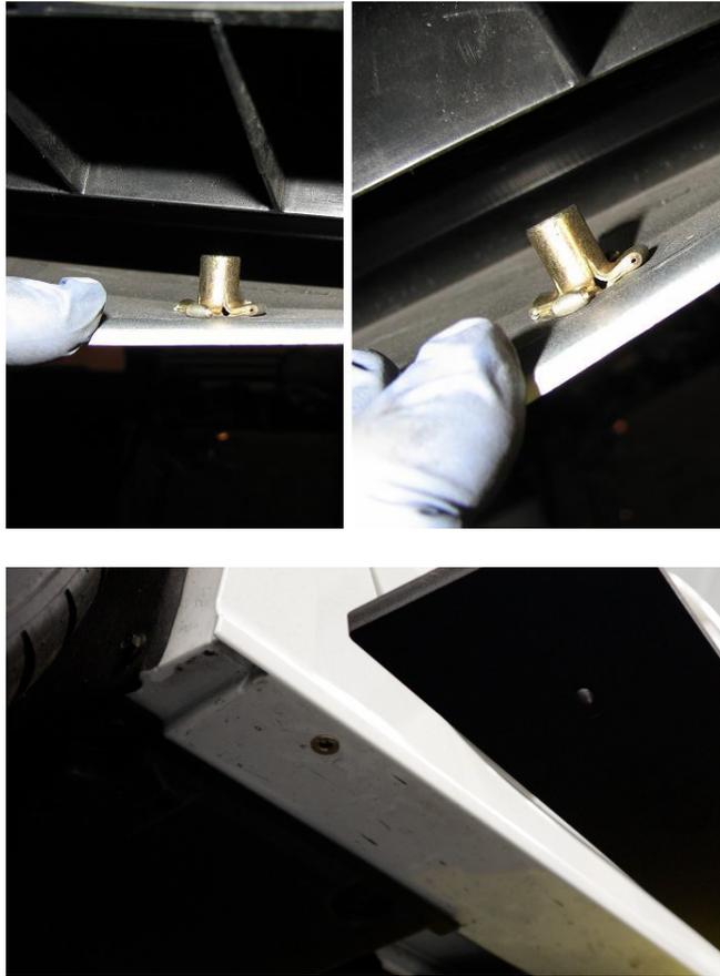
**2.12.** Once the rivet nuts are installed, loosely bolt the side splitter to the car using the supplied 35mm BHCS and large fender washers.
