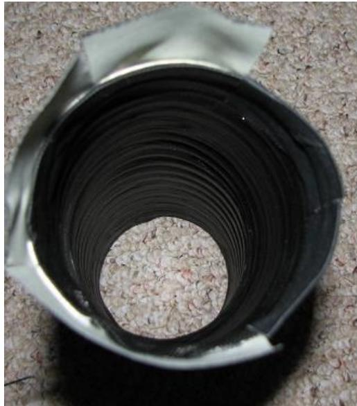
**2.30.3.** A fully finished duct is pictured below. The tape may not stick well to the hose due to the silicone/neoprene; however, once clamped it will hold well.
