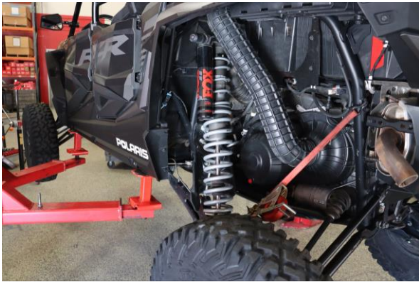
Step 21. Install the shock assembly into the vehicle.
