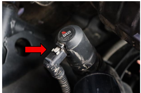
Step 24. Reconnect the shock electrical connector.
