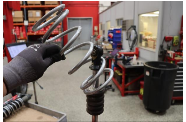
Step 16. Install the Eibach secondary spring.
