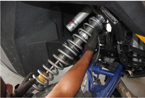
Step 15. Reinstall the coilover.
