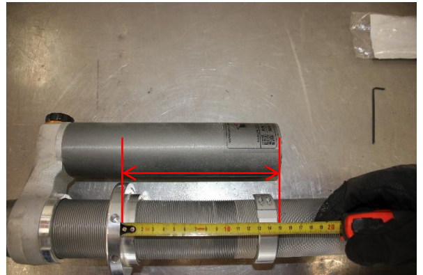
Step 10. Install the cross-over rings and set them at 120mm (4 3/4") measuring from the spring flange to the bottom of the crossover ring.
