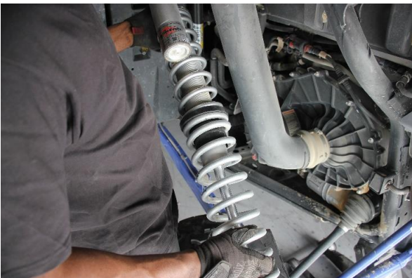
Step 17. Reinstall the coilover.
