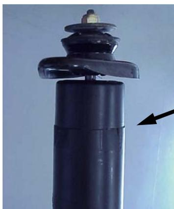
You must remove the rear shock, then, remove the upper mount to access the rear bump stop which is located underneath the OE dust boot
