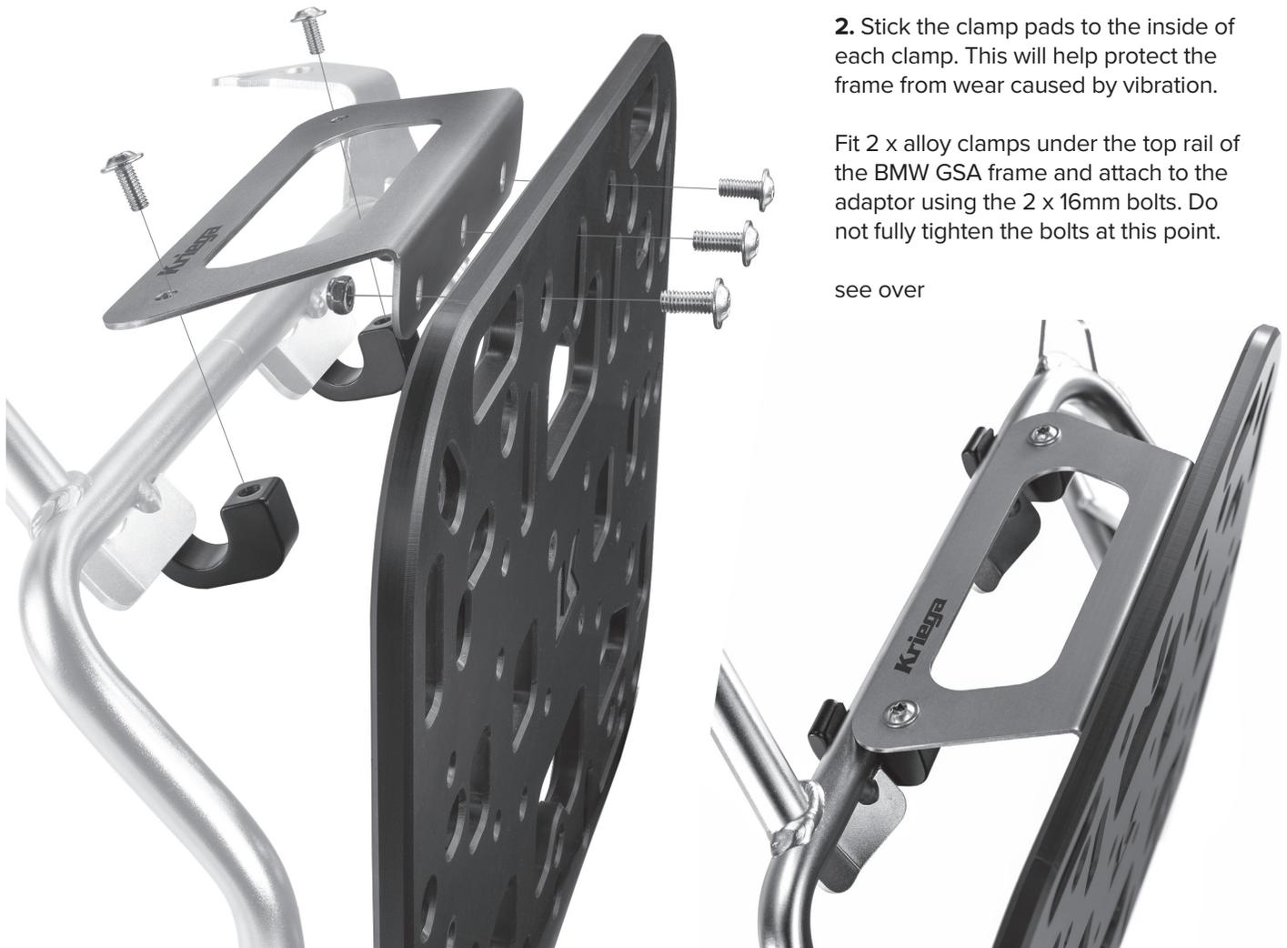
**3.** Fit the remaining 4 x alloy clamps in the positions as illustrated below. Once all clamps are in place and the OS-Platform is level with the frame you can fully tighten all the bolts. Use thread-lock on all bolts for extra safety.
