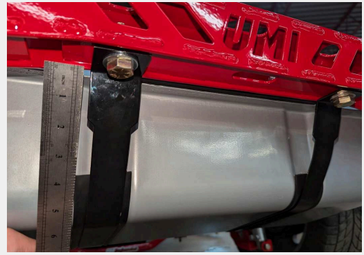
Figure 8: Measurement for tank strap bending
