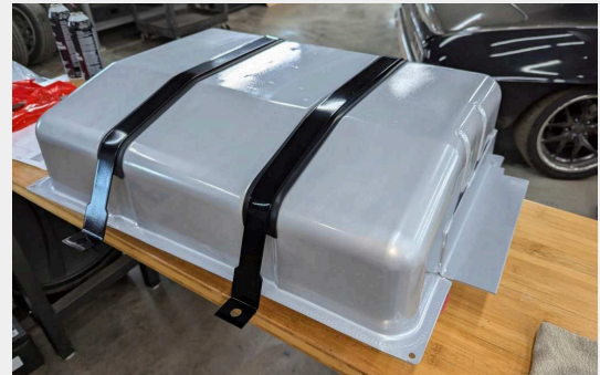
Figure 9: Tank straps bent around tank bottom
