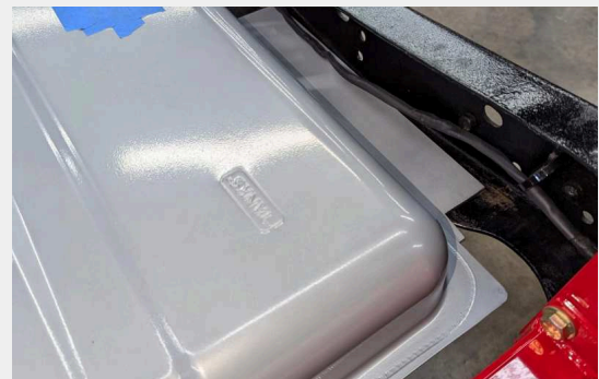
Figure 7: Side Flanges trimmed to allow better fitment under the crossmembers
