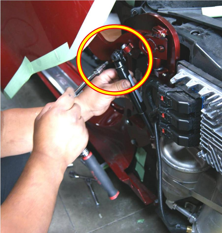
After installing the hinge and adjusting it, you can now install the shock.
