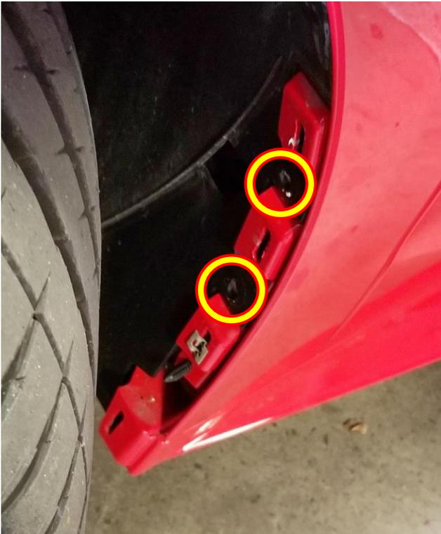
Remove the 3 screws (2 circled to the left 1 underneath) from the fender liner that way you can access the fender bolt.
