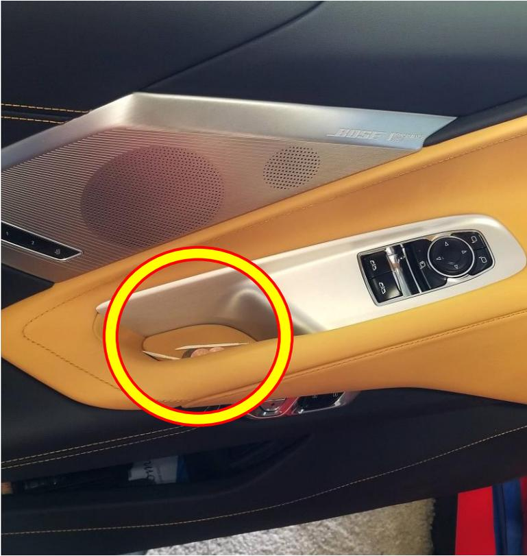
Remove the cover circled to the left with a plastic pry tool. (Remove any junk you have here first) You will then gain access to the bolts. Remove 2 bolts circled below.
