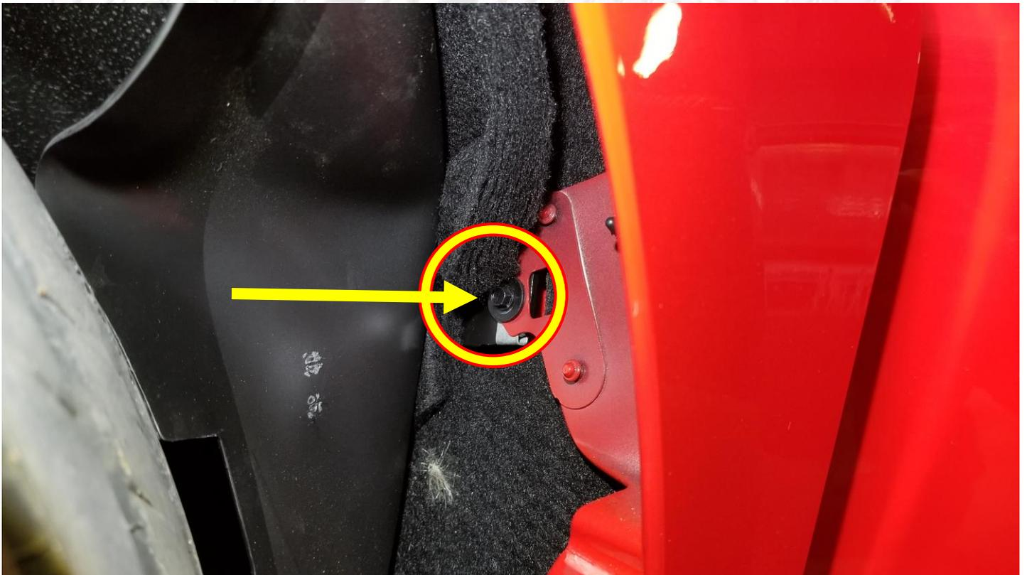
Remove 1 fender bolt (circled left) with the door open.
