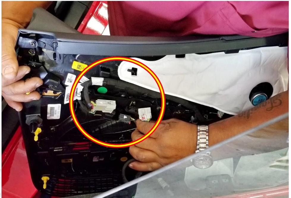
Remove the speaker by removing 4 screws. (Circled Below)
