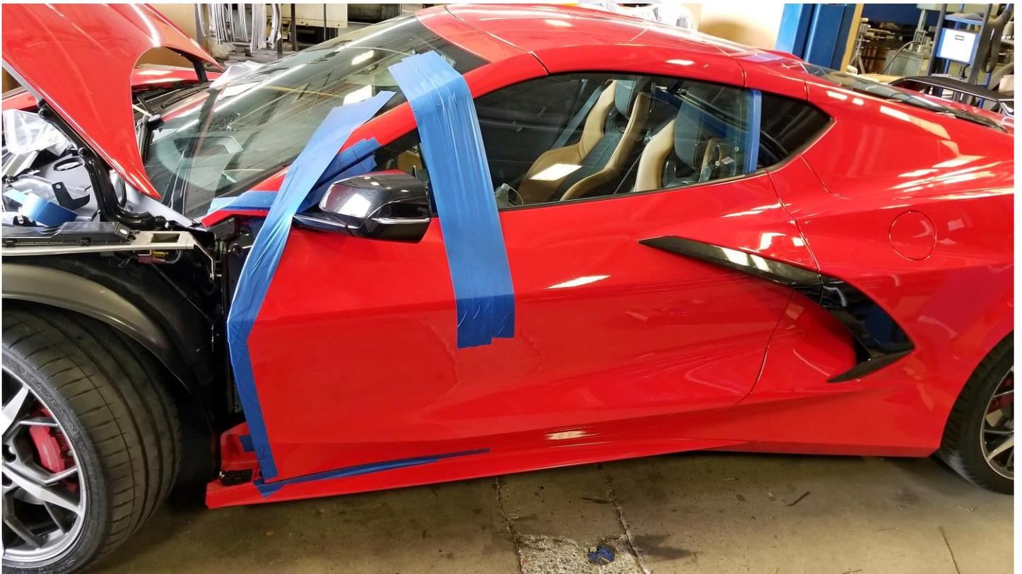
**Tip:** Cut a couple 3-inch pieces of paint stick to use as shims so the door does not move when you remove the factory hinges. Use them under and behind the door. Wrap them with painters' tape to get the exact thickness you need to shim the door.
