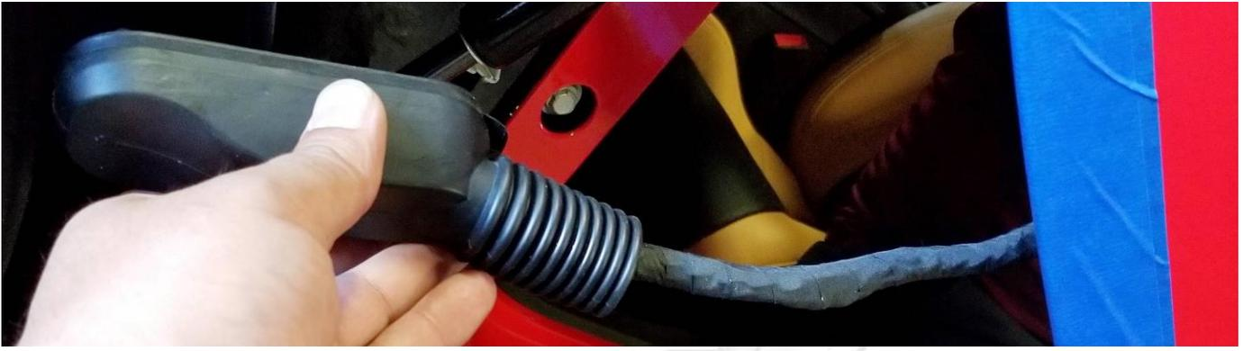
Cut the rubber wire boot in half as shown.
