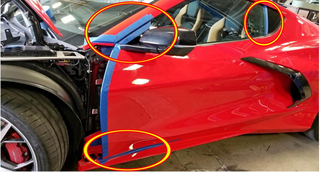
Use several strips of 2" painters' tape as shown to secure the door.
