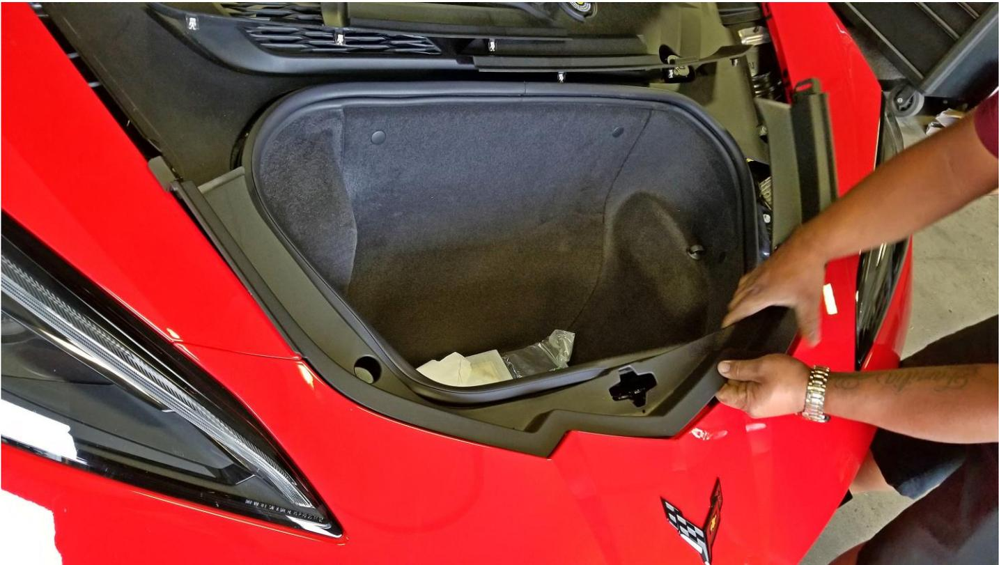
Now you can remove the panel covering the bumper bolts by pulling up on it to release clips
