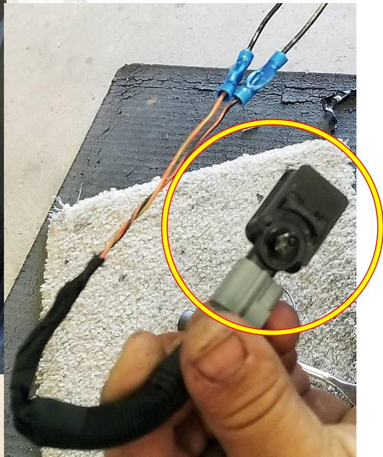
Wrap wires with a cloth tape for protection and flexibility. If you use regular electrical tape or you try to use loom the wires will bind up or pinch when you shut the door.
