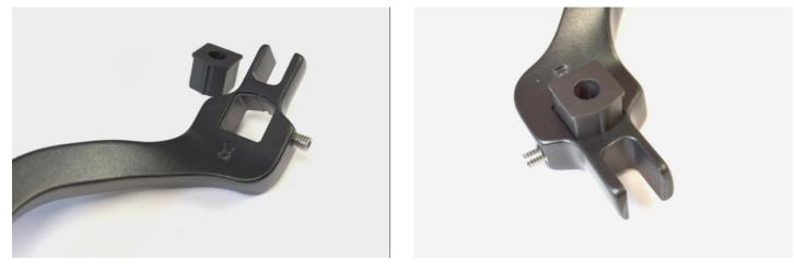
**STEP 4:** Now determine the best location of the handguard by moving it left or right to get the most coverage. The handguard should reach slightly beyond the end of the handlebars. **SEE PHOTO** Using 2 small spacers and 2 large spacers, position the handguard into the location you have chosen. **SEE PHOTO** Slide the long bolt through from the outside to the inside of the handguard and tighten with the lock nut. Position the handguard and now fully tighten the mounting bracket.
