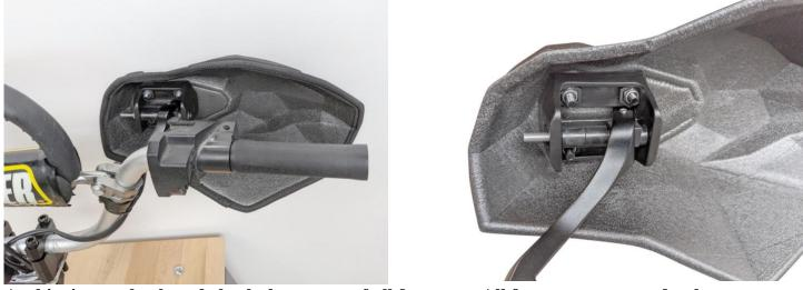
At this time go back and check the torque of all fasteners. All fasteners may need to be retightened after the first ride. Check the tightness of the bracket and handguard before each ride.
