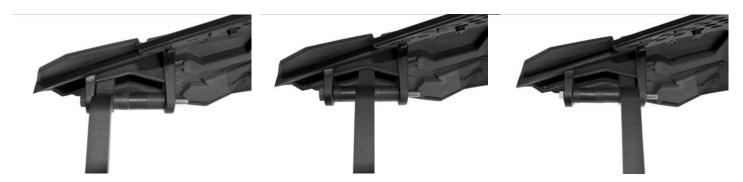
STEP 5: At this time go back and check the torque of all fasteners. All fasteners may need to be retightened after the first ride. Check the tightness of the bracket and handguard before each ride.
