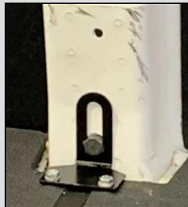
FLOOR IS DESIGNED TO FIT IN VANS AND ATTACH TO OEM MOUNTING POINTS WITHOUT DRILLING INTO THE VEHICLE
