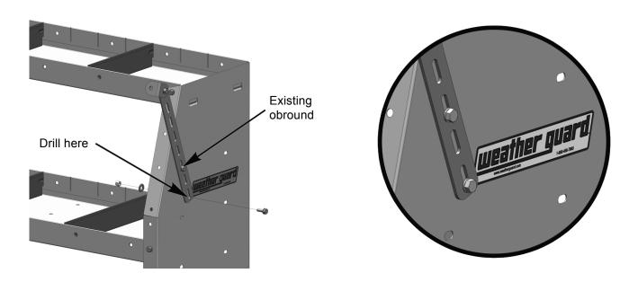
Install middle mounting point when possible. You can bend the mounting strap to create a triangular mounting to strengthen the shelf unit.
