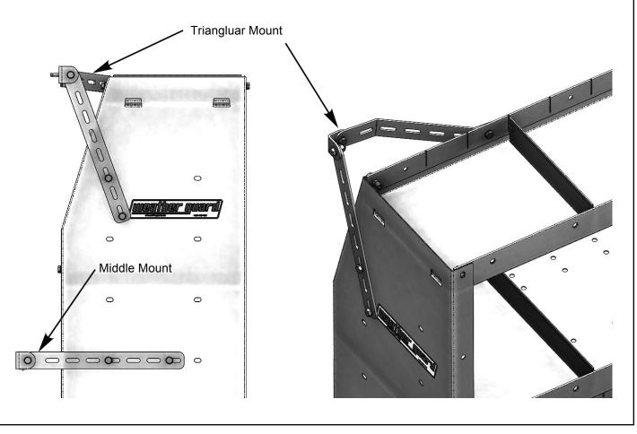
**STEP 9.** Verify the wall mounting locations and install blind fasteners. Existing holes may be used to install blind fasteners if they are located near the mounting straps. If not, they may still be used for ADDITIONAL mounting points using extra mounting straps. We recommend using two mounting angles on the strap joining two shelf units. One mounting foot can be shared between two shelf units.
