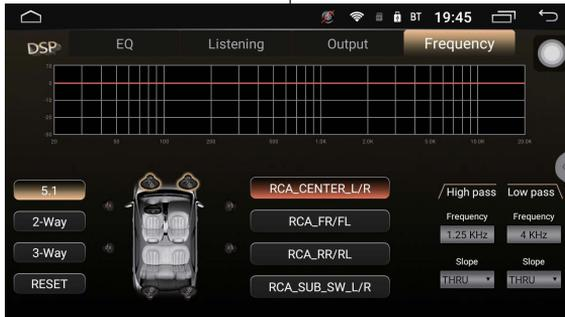
Frequency division supports 5.1, two frequency division and three frequency division for RCA speaker lines. The function of the reset button is used to reset parameters for adjusted parameters.
