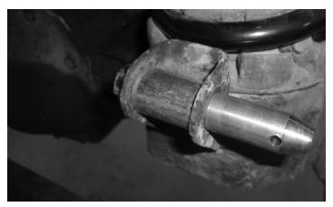
O Thread the tapered Stainless Steel Post (C) on to the 1/2" x 2-1/2" Bolt (K) from the outboard side of U-bracket and and tighten to 65 ft-lb. using a
