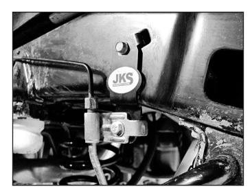
Cycle the suspension to full droop to ensure the brake lines have enough slack and clearance to the sway bar.
