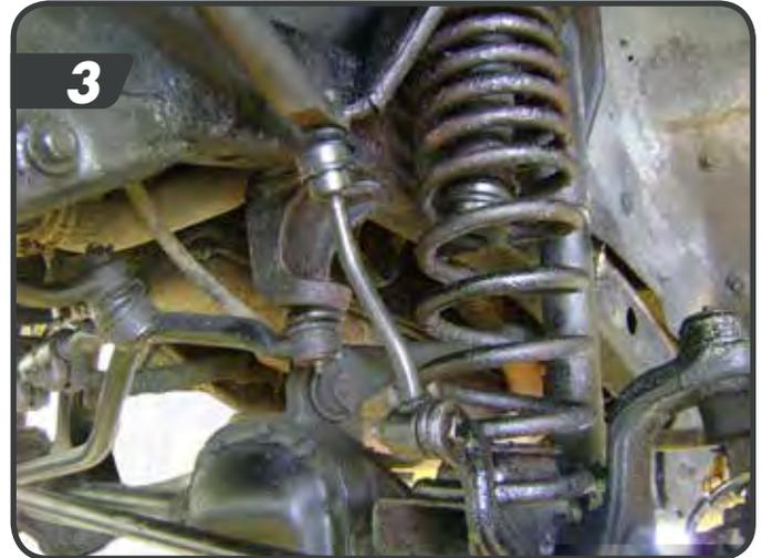
*Note: If difficult to remove the sway bar link from the sway bar, an air chisel or pickle fork can be used.*
