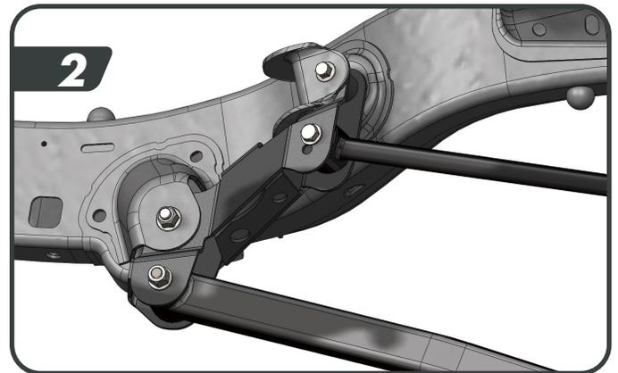
*Note: You may find it easier to align the control arms to the mount by removing the opposite side upper control arm and adjusting the axle with a hydraulic jack.*
