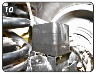
The shocks come with the bushings and upper spacers pre-installed. The wide mount will be installed up, at the frame. Slide the shock up into the mount. The longer shocks will be used in the rear. JSPEC shocks will be installed body down, Fox shocks will be installed body up.
