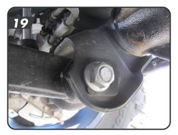
e. Repeat cam bolt installation on the driver's side.
