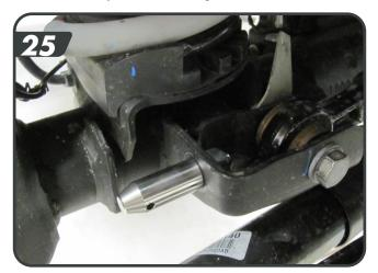
s. Install the longer disconnect post on the driver side axle sway bar link mount with it pointing inboard [26]. Fasten with the ½" nylock nut and tighten to 64 ft-lbs. Tighten the post with the pin hole parallel to the ground. Slide the polyurethane spacer on the pin up against the axle tab.
