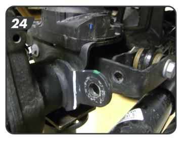
r. Install the shorter passenger side post on the side of the track bar mount at the sway bar link mount location with it pointing outboard [25]. Fasten with the ½" nylock nut and tighten to 64 ft-lbs.
