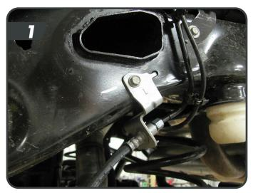
d. Remove the (2) bolts holding the TPMS ECU sensor to the rear crossmember (10mm) [2].
