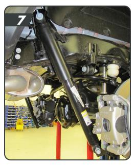
k. Lower the axle enough to remove the factory springs. Note the orientation of the upper spring isolators. Make sure there is adequate slack on all brake lines.
