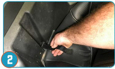
Using the (4) straps, secure the cooler bag to the vehicle at all corners of cooler bag. Bag will fit perfectly in the rear bed matching the shape and contour as shown. Cooler bag fits perfectly with our Multi-purpose bed storage bag (P199Y332).
