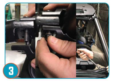
Running bolts through opposite clamps, tighten 2 bolts per clamp to hold each clamp in position. Make final adjustments and desired placement, then tighten firmly as your last step.
