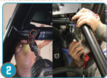
Running bolts through clamp, tighten 2 bolts per clamp to hold each clamp in position. Do not completely tighten until desired position and adjustments are completed.
