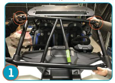
Place the intrusion bar over front of cage as shown, running bolts through upper clamp and hand tightening bolts to get you started and ease of install.
